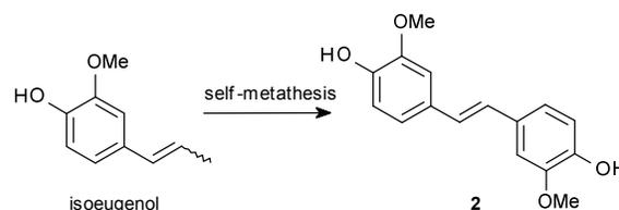
Scheme 2 Hitce's synthesis of 4,4'-dihydroxy-3,3'-dimethoxystilbene **2**.
