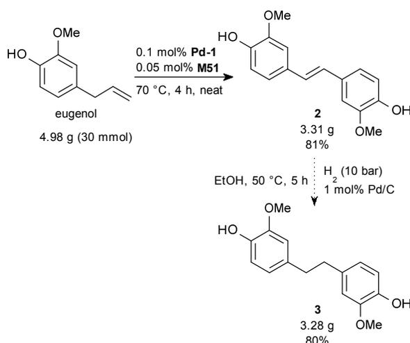
Scheme 3 Synthesis of di(hydroxyphenyl) derivatives from eugenol via isomerising metathesis and optional hydrogenation.
