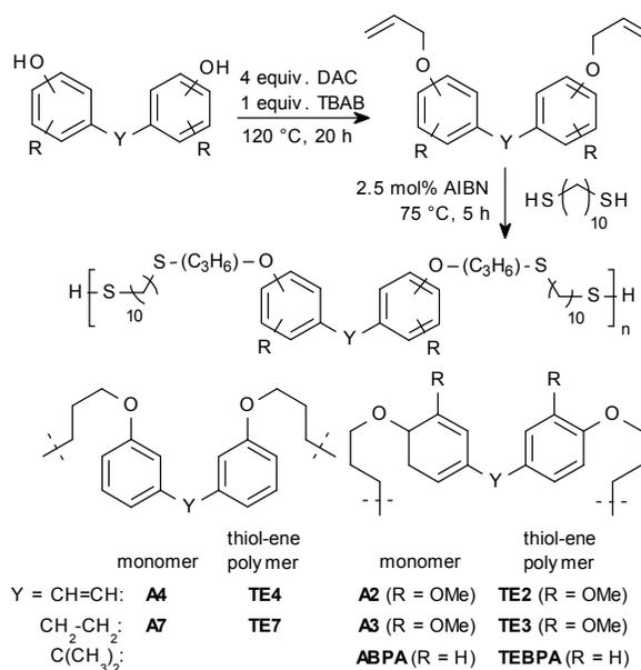
Scheme 6 Thiol-ene polymerisation. DAC = diallyl carbonate.
