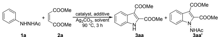
The reaction scheme shows the annulation of **1a** (N-phenylacetohydrazide) and **2a** (dimethyl maleate) to form **3aa** (2,3-dimethyl-1H-indole-5-carboxylate) and **3aa'** (2,3-dimethyl-1H-indole-5-carboxylate with an NHAc group). The reaction conditions are: catalyst, additive,  $\text{Ag}_2\text{CO}_3$ , solvent, 90 °C, 3 h.
