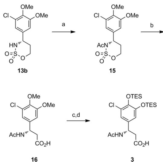
Scheme 3. Conversion of oxathiazinane **13b** into amino acid **16** and synthesis of amino acid building block **3**. a)  $\text{KOtBu}$ ,  $\text{AcCl}$ , THF, r.t., 8 h, 74 %; b) i)  $\text{MeCN}/\text{H}_2\text{O}$ , 50 °C, 4 h; ii) TEMPO,  $\text{NaOCl}$ ,  $\text{NaClO}_2$ , 35 °C, 16 h, 64 %; c)  $\text{AlBr}_3$ ,  $\text{EtSH}$ , 0 °C → r.t., 24 h; d) TESCl,  $\text{NEt}_3$ , DMAP, DMF, r.t., 8 h, 61 %, 2 steps.
