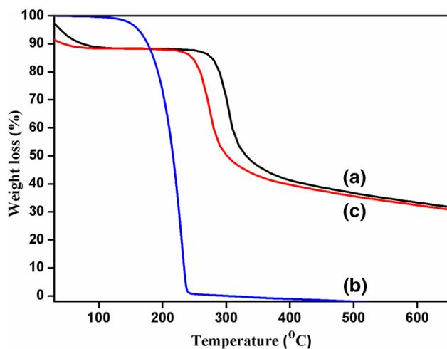
**Fig. 8** TGA of (a) chitosan, (b) vanillin and (c) C-FMPC-Nps
