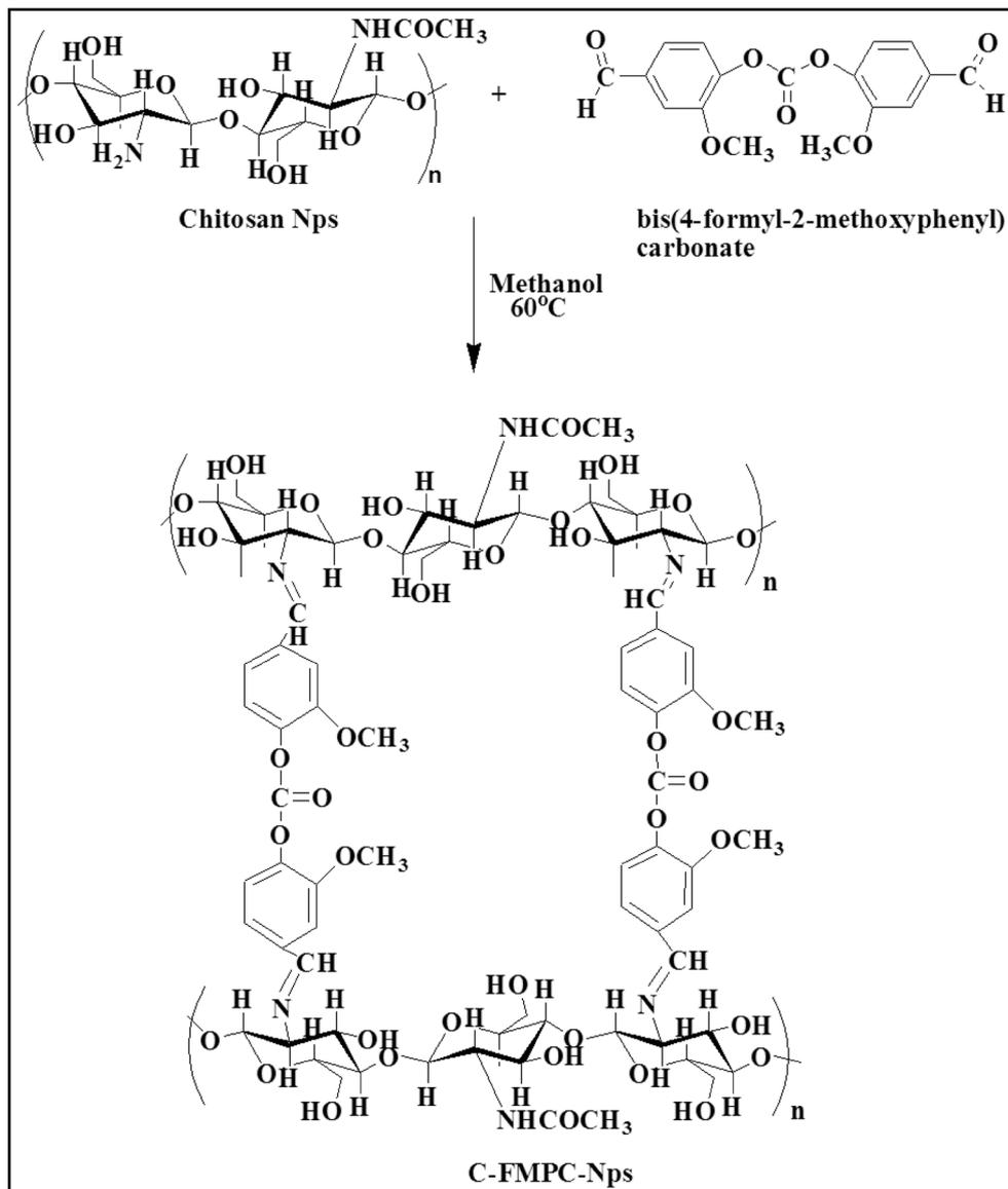
Scheme 2 Schematic structure of newly synthesized C-FMPC-Nps Schiff base
