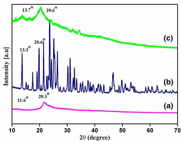
Fig. 7 XRD of (a) chitosan, (b) vanillin and (c) C-FMPC-Nps
