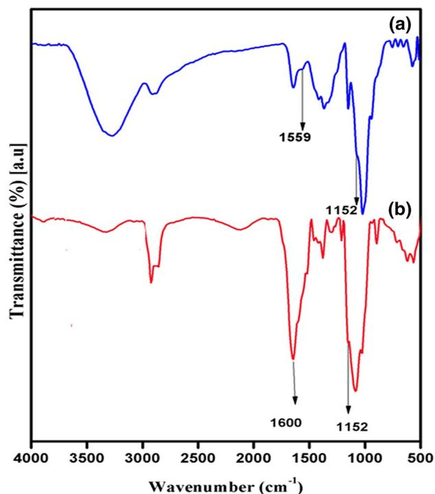
**Fig. 2** FTIR of (a) chitosan and (b) C-FMPC-Nps
