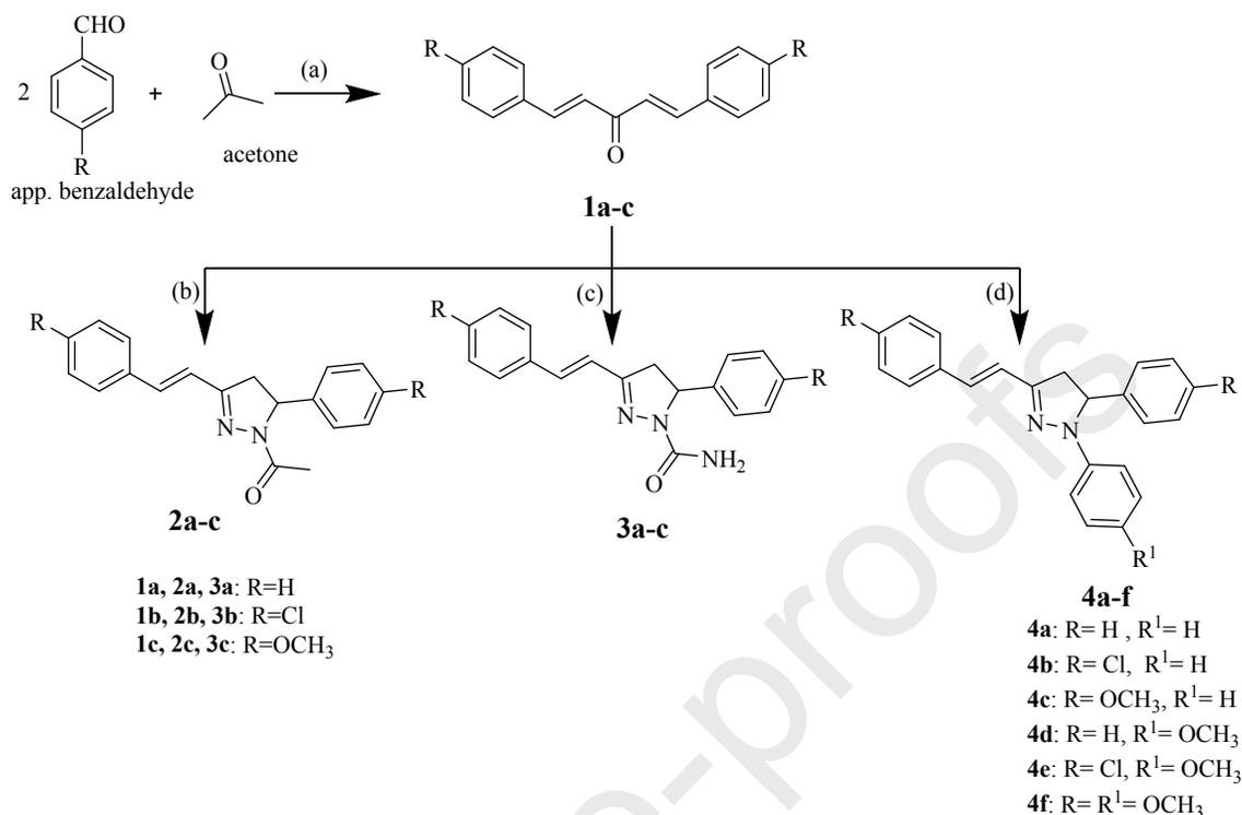
**Reagents and conditions:** (a) NaOH, absolute ethanol, RT, 1.5h; (b) Hydrazin hydrate, glacial acetic acid, 8h; (c) Semicarbazide.HCl, NaOH, EtOH, 8h; (d) Phenyl hydrazine, glacial acetic acid, EtOH, 8h or *p*-methoxy phenyl hydrazine HCl, EtOH, 8h.
