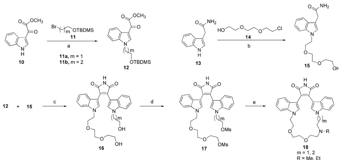
**Scheme 3.** (a)  $\text{Cs}_2\text{CO}_3$ , DMF, 50–75 °C, 68–82%; (b)  $\text{Cs}_2\text{CO}_3$ , DMF, 78 °C, 82%; (c) *t*-BuOK, THF, 0–23 °C; then concd HCl; (d)  $\text{Ms}_2\text{O}$ , pyridine, THF, 50 °C; (e) *i*-Pr<sub>2</sub>NEt, DMF, 90 °C, 11–20% overall from **15**.
