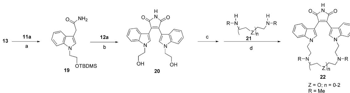
**Scheme 4.** (a) NaH, DMF, 60%; (b) *t*-BuOK, THF, 0–23 °C, then concd HCl, 83%; (c)  $\text{Ms}_2\text{O}$ , pyridine, THF, 50 °C, quantitative yield; (d) *i*-Pr<sub>2</sub>NEt, DMF, 100 °C, 15–30%.
