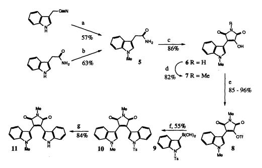
Scheme: (a) i. KOH, MeI, acetone; ii.  $H_2O_2$ ,  $K_2CO_3$ , DMSO; (b) NaH, MeI, DMF; (c) t-BuOK, MeOC(O)C(O)OMe, DMF; (d) NaH (2 equiv), MeI, DMF; (e) TEA, Tf<sub>2</sub>O, CH<sub>2</sub>Cl<sub>2</sub>; (f) Pd<sub>2</sub>dba<sub>3</sub>-CHCl<sub>3</sub>, CsF (3 equiv), CsBr (3 equiv), dioxane, 15 °C to rt; (g)  $K_2CO_3$ , MeOH/H<sub>2</sub>O.
