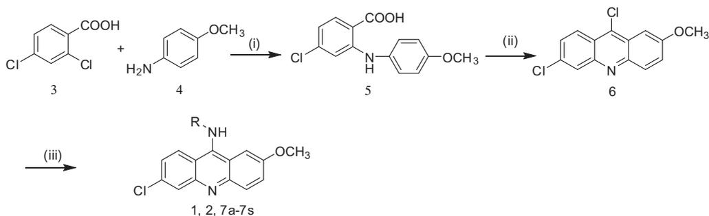
**Scheme 1.** Synthesis of the desired compounds (**1**, **2** and **7a–7s**). Reagents and conditions: (i) K<sub>2</sub>CO<sub>3</sub>, Cu, DMF, 130 °C; (ii) POCl<sub>3</sub>, 140 °C; (iii) various anilines/amines, for **1**, **2** and **7a–7n** CHCl<sub>3</sub>, EtOH, concd HCl, for **7o–7s** DMF, KI, NaH.
