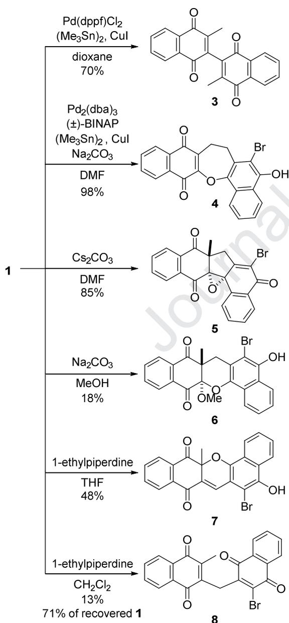
**Scheme 1.** Previous dimerizations of 2-bromo-3-methyl-1,4-naphthoquinone (**1**).
