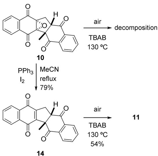
**Scheme 6.** Reactions of **10** and **14** in TBAB under an aerobic atmosphere.
