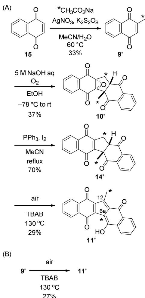
**Scheme 7.** Synthesis of  $^{13}\text{C}$ -labeled 1-methylKuQuinone **11'** from 1,4-naphthoquinone (**15**) (A) and via dimerization of 2-(methyl- $^{13}\text{C}$ )-1,4-naphthoquinone (**9'**) (B).
