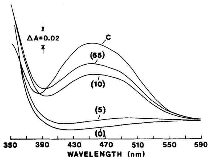
FIG. 6. Spectra of DHLA-reduced CG 8-935. The reaction mixture contained 50 mM potassium-phosphate, pH 7.4, and 50  $\mu$ M CG 8-935. C, unreduced CG spectrum. Reduction was started by adding 300  $\mu$ M DHLA. The figures in parentheses indicate the time (min) elapsed after adding DHLA. Scanning velocity, 2 nm/sec. Other conditions were as described under Materials and Methods.
