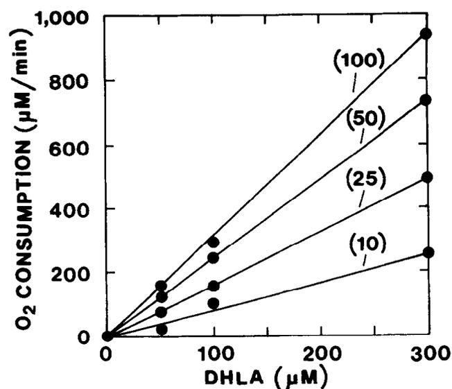
FIG. 5. Effect of DHLA and CG 8-935 concentrations on the rate of oxygen consumption. Experimental conditions were as described in the legend of Fig. 2, except for DHLA and quinone concentrations, which are indicated on the abscissa and by figures in parentheses ( $\mu\text{M}$ ), respectively.
