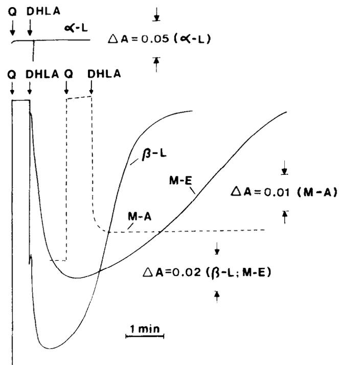
FIG. 13. Kinetics of  $\beta$ -lapachone ( $\beta$ -L), mansonone A (M-A), mansonone E (M-E) and  $\alpha$ -lapachone ( $\alpha$ -L) redox-cycling in the presence of DHLA and SOD. The reaction mixture contained 50 mM potassium-phosphate, pH 7.4, 20 U/mL of SOD, and 50  $\mu$ M quinone (Q) as indicated near the tracings. The reaction was started by adding 50  $\mu$ M DHLA as indicated by the arrows. Absorbance was measured at 450 nm. Other conditions were as described under Materials and Methods.
