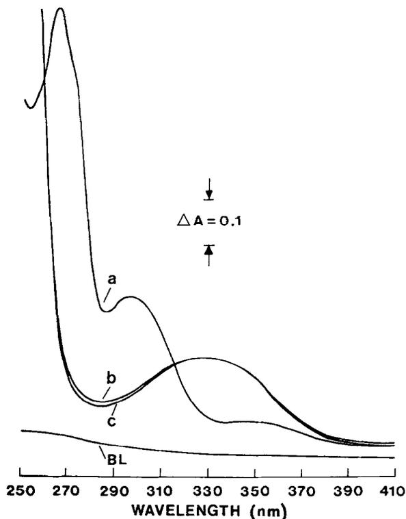
FIG. 3. Spectra of CG 8-935 and DHLA-reduced quinone. The reaction mixture contained 50 mM potassium-phosphate buffer, pH 7.4, and 40  $\mu\text{M}$  CG 8-935. Key: (a) control spectrum; (b) same as (a) with addition of 300  $\mu\text{M}$  DHLA; (c) same as (b) with addition of 800  $\mu\text{M}$  borohydride. Spectra (b) and (c) were recorded immediately after reductant addition. BL, base line. Slit, 30 nm. Scanning velocity, 2 nm/sec.
