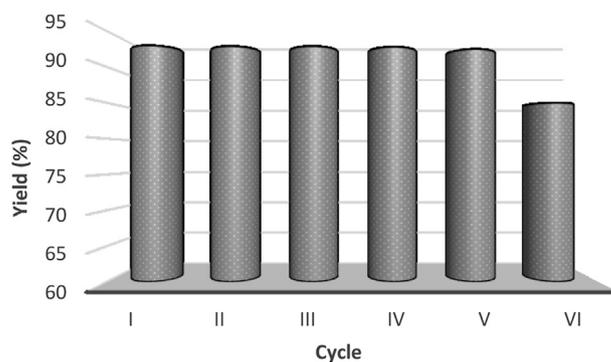
**Fig. 1.** Catalyst activity for six cycles.
