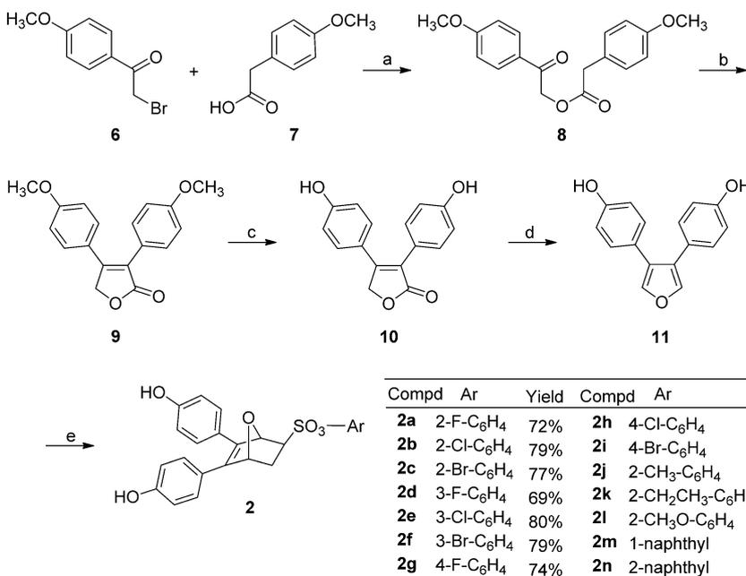
**Scheme 3.** Synthesis of oxabicycloheptene sulfonate derivatives **2a–n** using an improved procedure. Reagents and conditions: a) Et<sub>3</sub>N, CH<sub>3</sub>CN, RT, 88%; b) NaH, DMSO, 25 °C, 75%; c) BBr<sub>3</sub>, CH<sub>2</sub>Cl<sub>2</sub>, –78 °C → RT, 85%; d) DIBAL-H, THF, –78 °C, 71%; e) **5** (neat), 90 °C.
