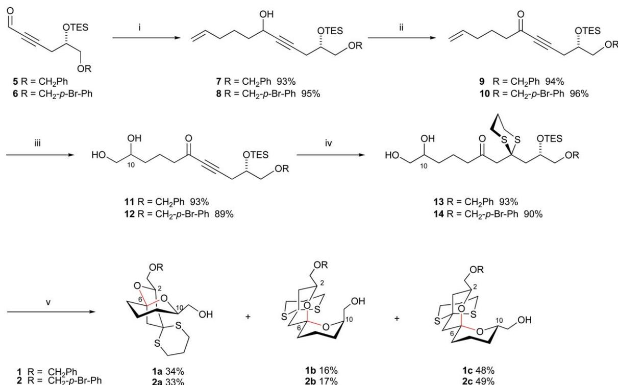
**Scheme 3** Reagents and conditions: (i) CH<sub>2</sub>=CH(CH<sub>2</sub>)<sub>3</sub>MgBr, Et<sub>2</sub>O, 30 °C, 4 h; (ii) Dess–Martin periodinane, DCM, rt, 2 h; (iii) OsO<sub>4</sub>, NMO, H<sub>2</sub>O–*t*-BuOH, 0 °C, 18 h; (iv) HS(CH<sub>2</sub>)<sub>3</sub>SH, NaOMe, MeOH–DCM, -10 °C, 18 h; (v) HClO<sub>4</sub> 10% aq., MeCN–DCM, 0 °C, 30 min.
