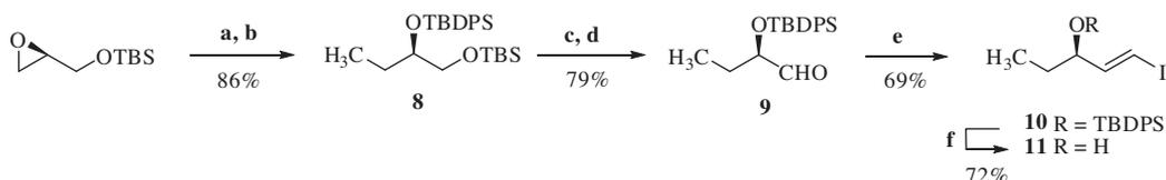
**Scheme 3.** Synthesis of C16–C20 fragment. Reagents and conditions: (a)  $\text{CH}_3\text{MgBr}$ , CuI, THF, –78 °C, 2 h; (b) TBDPSCl, DMAP, imidazole,  $\text{CH}_2\text{Cl}_2$ , 17 h; (c) CSA, MeOH,  $\text{CH}_2\text{Cl}_2$ , 0–5 °C, 3 h; (d)  $\text{Pyr-SO}_3$ , DMSO,  $\text{Et}_3\text{N}$ ,  $\text{CH}_2\text{Cl}_2$ , 0 °C, 3 h; (e)  $\text{CrCl}_2$ ,  $\text{CH}_2\text{Cl}_2$ , THF, 0 °C to rt, 1 h; (f) TBAF, THF, 0 °C, 2 h.
