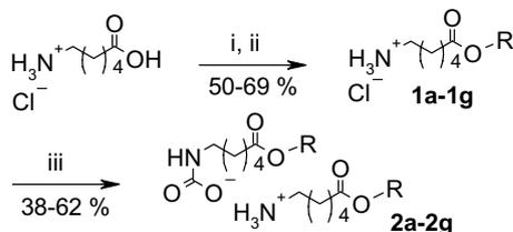
**Scheme 2.** Synthesis of the branched carbamate salts. Reagents and conditions (i)  $\text{SOCl}_2$ ,  $40^\circ\text{C}$ , 30 min; (ii):  $\text{R-OH}$ ,  $\text{CHCl}_3$ , reflux, 1.5 h; (iii): TEA,  $\text{CO}_2$ . R: as in Figure 1.
