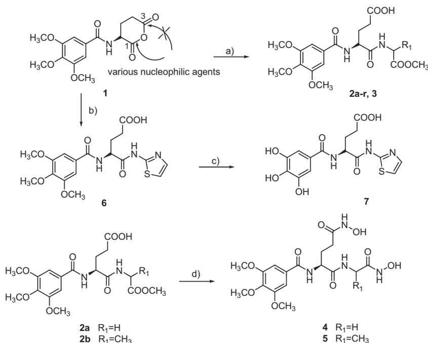
Reagents and conditions: a) Various L-amino acid methyl ester hydrochloride, anhydrous CH<sub>2</sub>Cl<sub>2</sub>, Et<sub>3</sub>N, rt. b) thiazol-2-amine, acetic acid, rt. c) BBr<sub>3</sub>, CH<sub>2</sub>Cl<sub>2</sub>, DMF, 0°C. d) NH<sub>2</sub>OK in anhydrous CH<sub>3</sub>OH, then acetic acid (two steps).
