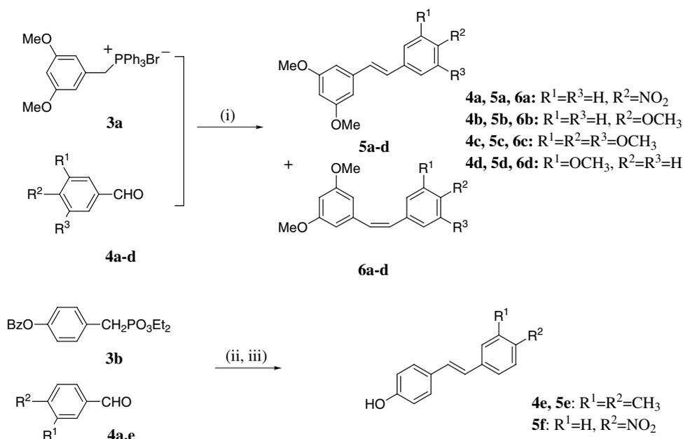
**Scheme 1.** Reagents and conditions: (i) **3a** (1.1 equiv), **4a–d** (1 equiv), NaH (1.2 equiv), THF, 4–16 h, room or reflux temperature, 30–50% yield, 1:1 to 1:3 *Z/E* isomer ratio; (ii) same conditions as (i), but only *E*-isomers were recovered; (iii) AlCl<sub>3</sub>, *N,N*-dimethylaniline, CH<sub>2</sub>Cl<sub>2</sub>, rt, 60% yield.
