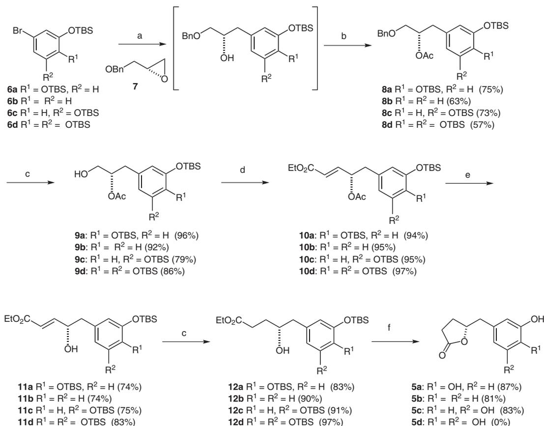
**Scheme 1** Reagents and conditions: (a) BuLi, THF then **7**, BF<sub>3</sub>·OEt<sub>2</sub>, THF, -78 °C to r.t.; (b) Ac<sub>2</sub>O, Et<sub>3</sub>N, DMAP, CH<sub>2</sub>Cl<sub>2</sub>; (c) H<sub>2</sub>, 10% Pd/C, EtOAc; (d) (ClCO)<sub>2</sub>, DMSO, Et<sub>3</sub>N, CH<sub>2</sub>Cl<sub>2</sub> then Ph<sub>3</sub>P=CHCO<sub>2</sub>Et; (e) K<sub>2</sub>CO<sub>3</sub>, EtOH; (f) TsOH·H<sub>2</sub>O, 4 Å MS, benzene, reflux.
