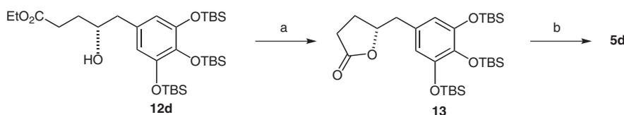
**Scheme 2** Reagents and conditions: (a) PPTS, benzene, reflux, 1 h, 98%; (b) concd HCl, THF–MeOH (5:1), 0 °C to r.t., 6 h, 81%.
