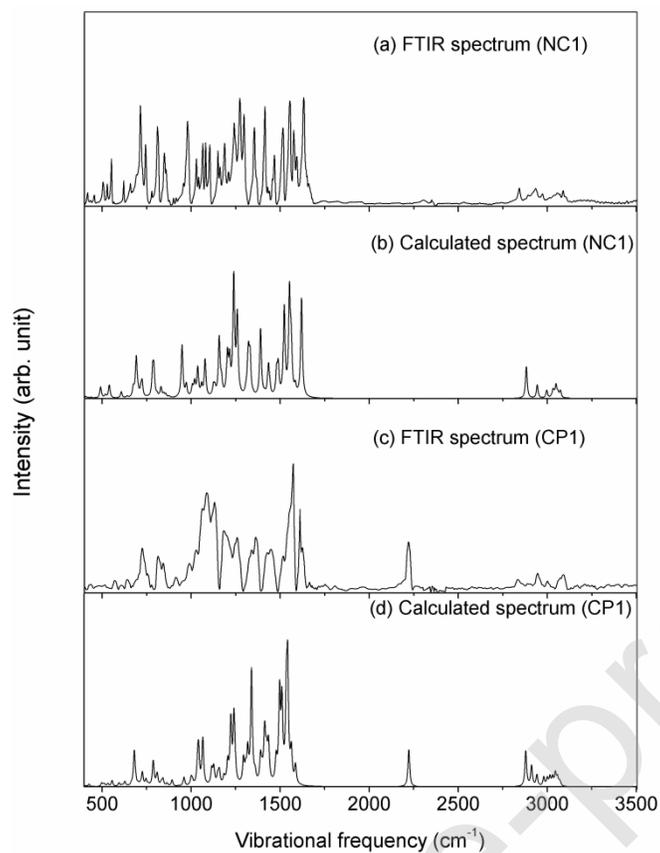
**Figure 2:** (a) FTIR spectrum of NC1 (b) calculated infrared spectrum of NC1 (c) FTIR spectrum of CP1 and (d) Calculated infrared spectrum of CP1. The calculated spectra were obtained with B3LYP/6-311++G(d,p) theory level. The calculated harmonic frequencies are scaled with a factor of 0.956.
