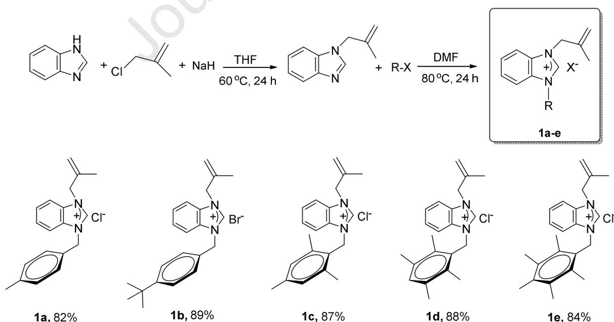
**Scheme 1.** Synthesis of benzimidazole-based ligand precursors (**1a-e**)
