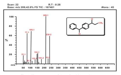
Fig. 6. Mass spectrum of 4-propionyl benzophenone
