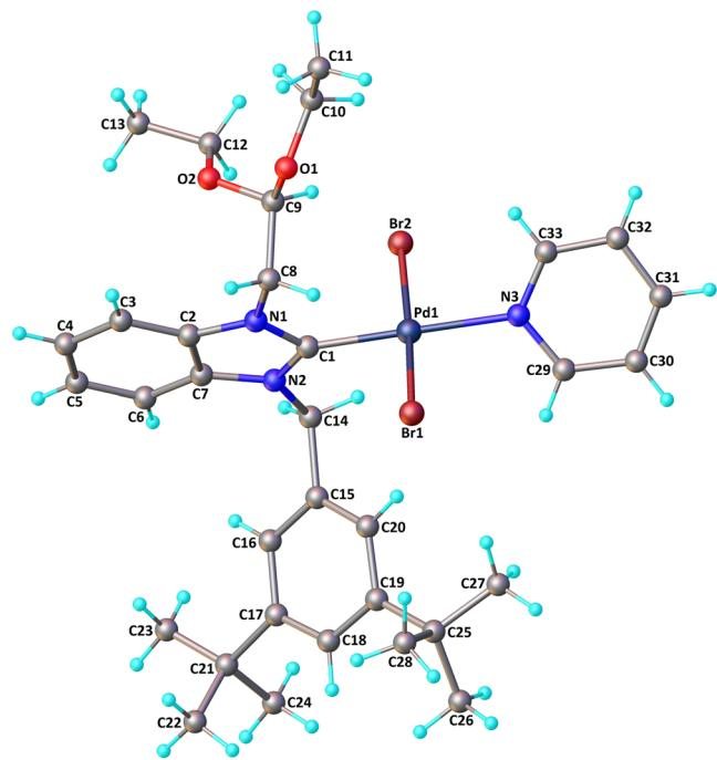
**FIGURE 5** Molecular structure of **3f** showing the atom numbering scheme. For the sake of clarity, only molecule A is shown.
