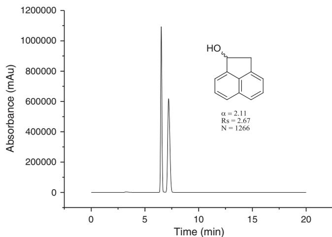
**Fig. 4.** Enantioselective separation of racemic 1-acenaphthenol on Chiralpak ID (4.6 mm ID, 250 mm length). Mobile phase: *n*-hexane/2-propanol 90:10 v/v, UV: 254 nm, flow rate: 1 mL/min.
