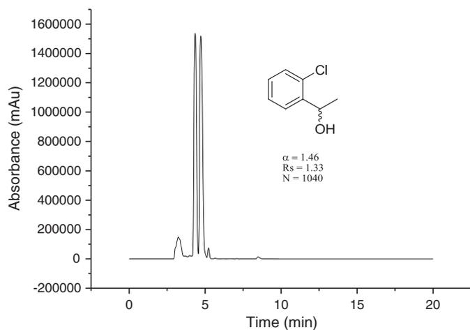
**Fig. 5.** Enantioselective separation of racemic 1-(2-chlorophenyl)ethanol on Chiralpak ID (4.6 mm ID, 250 mm length). Mobile phase: *n*-hexane/2-propanol 90:10 v/v, UV: 254 nm, flow rate: 1 mL/min.
