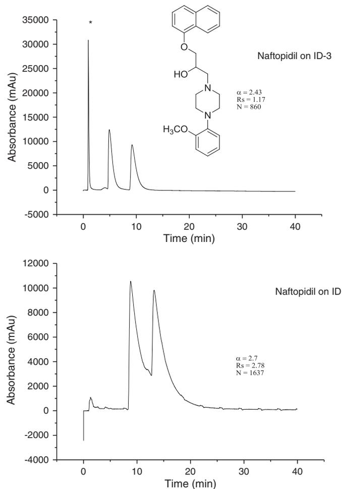
**Fig. 9.** Enantioselective separation of racemic naftopidil on the capillary (top) vs. the conventional Chiralpak ID (bottom). Mobile phase: *n*-hexane/2-propanol 90:10 v/v, UV: 219 nm, flow rate: 50  $\mu$ L/min and 1 mL/min, respectively. \*2-propanol.
