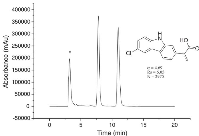
**Fig. 3.** Enantioselective separation of racemic carprofen on Chiralpak ID (4.6 mm ID, 250 mm length). Mobile phase: *n*-hexane/2-propanol 90:10 v/v, UV: 220 nm, flow rate: 1 mL/min. \*2-propanol.
