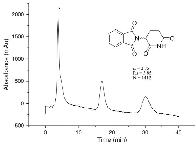
**Fig. 7.** Enantioselective separation of racemic thalidomide on Chiralpak ID-3 (0.3 mm ID, 150 mm length). Mobile phase: *n*-hexane/2-propanol 30:70 v/v, UV: 219 nm, flow rate: 10  $\mu$ L/min. \*2-propanol.
