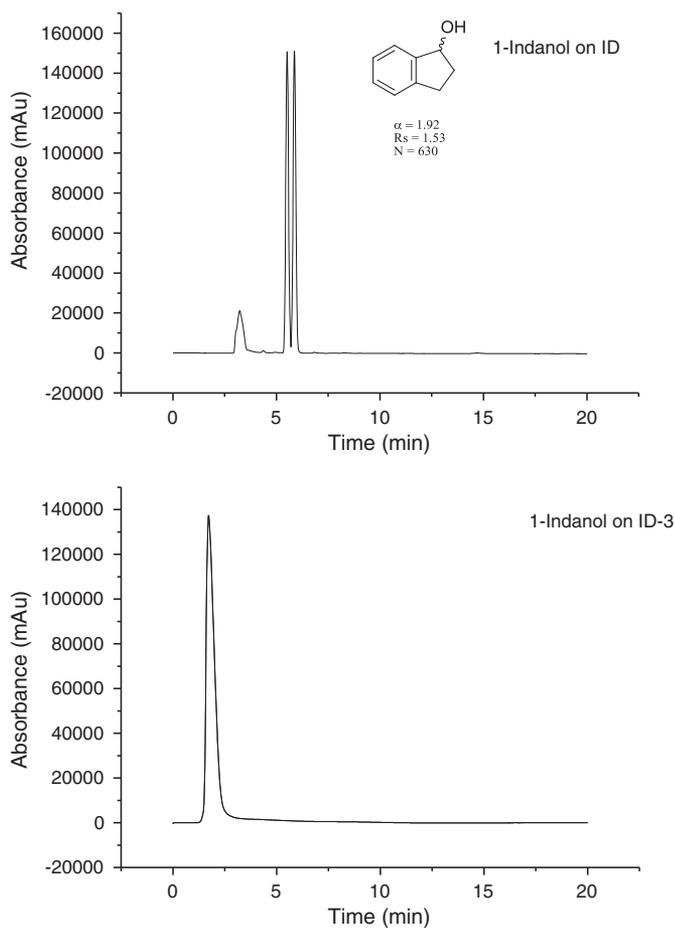
**Fig. 8.** Enantioselective separation of racemic 1-indanol on the conventional Chiralpak ID (top) vs. the capillary Chiralpak ID-3 (bottom). Mobile phase: *n*-hexane/2-propanol 90:10 v/v, UV: 254 nm, flow rate: 1 mL/min and 10  $\mu$ L/min, respectively.
