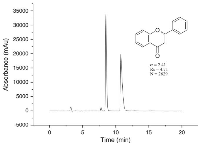
**Fig. 2.** Enantioselective separation of racemic flavanone on Chiralpak ID (4.6 mm ID, 250 mm length). Mobile phase: *n*-hexane/2-propanol 90:10 v/v, UV: 254 nm, flow rate: 1 mL/min.
