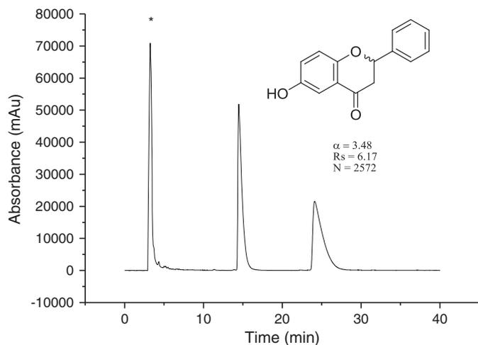
**Fig. 6.** Enantioselective separation of racemic 6-hydroxyflavanone on Chiralpak ID (4.6 mm ID, 250 mm length). Mobile phase: *n*-hexane/2-propanol 90:10 v/v, UV: 254 nm, flow rate: 1 mL/min.
