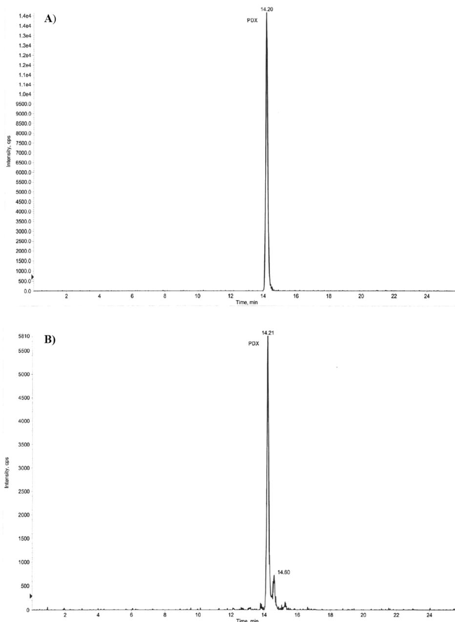
**Figure 3.** Comparison of LC–MS/MS profiles. Multiple reaction monitoring chromatograms for selected ion pair  $m/z$  359–206 of PDX (**2**) from Cayman Chemical Company (A) and synthetic compound (B).
