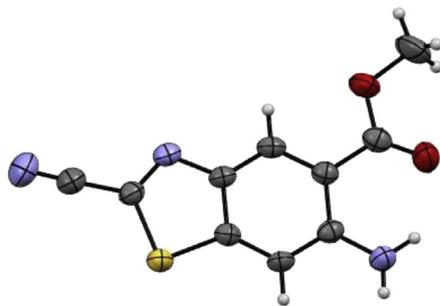
Fig. 2. ORTEP diagram of **1** (for details, see Experimental section and additional data).
