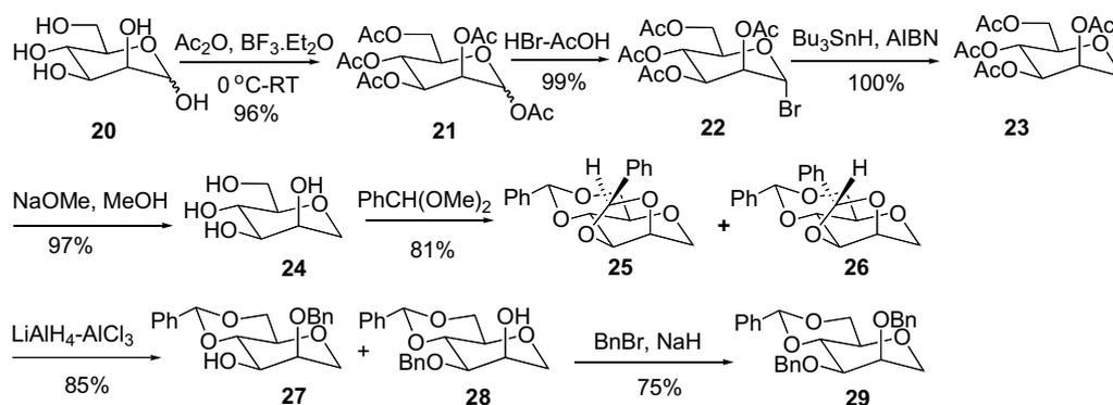
Scheme 1. Preparation of the protected 1,5-anhydro-D-mannitol intermediate **29**.
