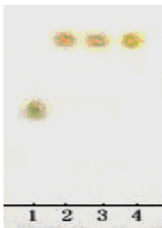
Fig. 4. A thin-layer chromatogram of dioscin by the dioscin- \alpha -L-rhamnosidase. The reaction mixture containing 0.1 mL of the substrate and 0.1 mL of the enzyme was incubated for 24 h at 42 °C. Lane 1: standard dioscin; Lane 2: standard diosgenyl- O - \beta -D-glucopyranoside; Lanes 3 and 4: two times products from enzymatic transformation.
