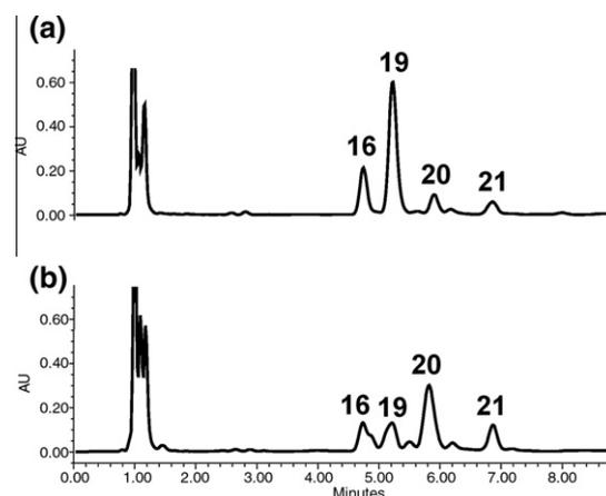
**Figure 1.** HPLC trace after (a) 50 min and (b) 100 min of reaction for the glycosylation of disaccharide acceptor **16** with donor **17** (5 equiv) activated with 2 equiv of  $\text{BF}_3 \cdot \text{OEt}_2$  at rt.
