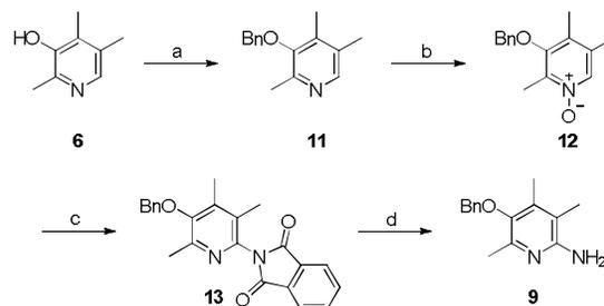
**Scheme 2.** An alternative synthesis of 6-amino-3-benzyloxy-2,4,5-trimethylpyridin-3-ol (**9**). *Reagents and conditions:* (a) PhCH<sub>2</sub>Cl, K<sub>2</sub>CO<sub>3</sub>, DMF, r.t., 12 h, 71%; (b) *m*-CPBA, CH<sub>2</sub>Cl<sub>2</sub>, r.t., 1 h, 94%; (c) *p*-TsCl, *i*-Pr<sub>3</sub>NEt, phthalimide, CH<sub>2</sub>Cl<sub>2</sub>, r.t., 12 h, 70%; (d) H<sub>2</sub>NNH<sub>2</sub>, THF-EtOH, r.t., 1 h, 90%.
