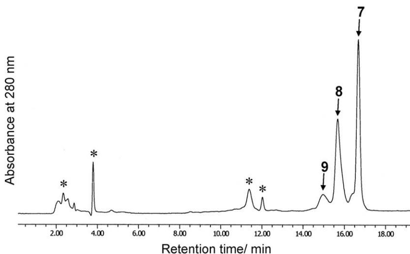
**Figure 2.** RP-HPLC profile of the Endo-M transglycosylation reaction. The transglycosylation to tri-GlcNAc insulin 7 at the reaction time of 8 h detected by the absorbance at 280 nm. \*: Impurity from SGP.
