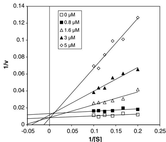
**Figure 2.** Double reciprocal plot of heparanase inhibition by sulfated pentasaccharide **15**. Heparanase assays were conducted at 0.9 μg/mL heparanase, various concentrations of [<sup>3</sup>H]HS, 40 mM sodium acetate, pH 5.0, and 0.1 mg/mL BSA at 37 °C for 4 h.
