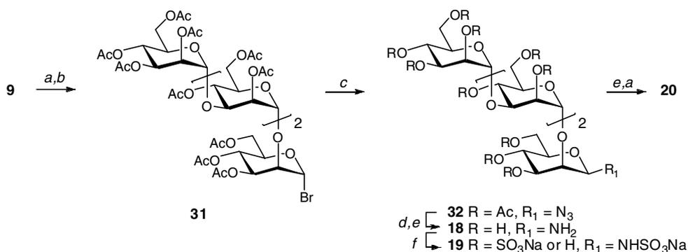
**Scheme 2.** Synthesis of tetrasaccharylamine derivatives **19** and **20**. Reagents and conditions: (a) Ac<sub>2</sub>O, Py, DMAP, rt, o/n; (b) HBr/HOAc/1,2-DCE, rt, o/n; (c) NaN<sub>3</sub>, DMF, 110 °C, o/n, 41% two steps; (d) NaOMe, MeOH, rt, 4 h, 72%; (e) PtO<sub>2</sub>, H<sub>2</sub> (100 psi), MeOH/EtOAc/AcOH, 3 h; (f) i—SO<sub>3</sub>·Py, DMF, 60 °C, 6 h; ii—1 M NaOH, 55% two steps.
