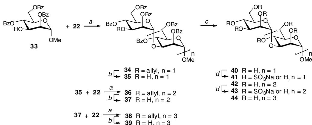
**Scheme 3.** Synthesis of all  $\alpha(1 \rightarrow 3)$ -linked mannoooligosaccharides. Reagents and conditions: (a) TMSOTf, 1,2-DCE, 0 °C  $\rightarrow$  rt, 30 min; (b) PdCl<sub>2</sub>, MeOH/1,2-DCE, 70 °C, 40 min, 54–70%, two steps; (c) NaOMe, MeOH/THF, rt, o/n, 85–98%; (d) i—SO<sub>3</sub>Py, DMF, 60 °C, 6 h; ii—1 M NaOH, 36–48%.
