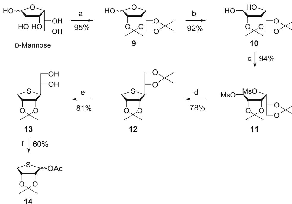
**Reagents and Conditions:** a) 2,2-dimethoxypropane, camphosulfonic acid, acetone, rt, 15 h; b) NaBH<sub>4</sub>, EtOH, rt, 2 h; c) MsCl, Et<sub>3</sub>N, CH<sub>2</sub>Cl<sub>2</sub>, rt, 1 h; d) Na<sub>2</sub>S, DMF, 80 °C, 15 h; e) 60% AcOH, rt, 2 h; f) Pb(OAc)<sub>4</sub>, EtOAc, rt, 15 h.
