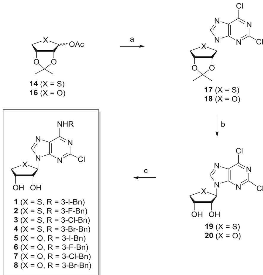
**Reagents and Conditions:** a) 2,6-dichloropurine, HMDS,  $(\text{NH}_4)_2\text{SO}_4$ , TMSOTf,  $\text{ClCH}_2\text{CH}_2\text{Cl}$ , 0 to 80 °C, 2 h; b) 1 N HCl, rt, 15 h; c) 3-halobenzylamine, EtOH, rt, 2 h - 3 d.
