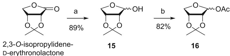
**Reagents and Conditions:** a) DIBAL, toluene, -78 °C, 30 min; b) Ac<sub>2</sub>O, pyridine, rt, 3 h.
