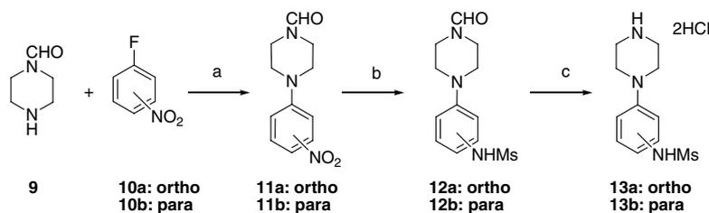
**Scheme 2.** Reagents and conditions: (a)  $K_2CO_3$ , DMSO, 50 °C, 1 h, 88% for **11a**, 89% for **11b**; (b) i— $H_2$ , 10% Pd/C, EtOH, THF, rt, 14 h; ii—MsCl,  $Et_3N$ , THF, 0 °C, 1 h, 73% for **12a**, 80% for **12b**; (c) 2 N methanolic HCl, 50 °C, 1 h, 76% for **13a**, 92% for **13b**.
