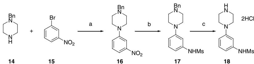
**Scheme 3.** Reagents and conditions: (a)  $Pd_2(dba)_3$ , BINAP, *t*-BuONa, toluene, 90 °C, 5 h, 36%; (b) i—Fe,  $NH_4Cl$ ,  $H_2O$ , MeOH, 100 °C, 3 h; ii—MsCl,  $Et_3N$ , THF, 0 °C, 1 h, 91% over 2 steps; (c)  $H_2$ , 20%  $Pd(OH)_2/C$ , 2 N methanolic HCl, rt, 14 h, 63%.
