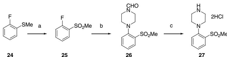
**Scheme 6.** Reagents and conditions: (a)  $H_2O_2$ , AcOH,  $Na_2WO_4 \cdot 2H_2O$ , 80 °C, 5 h, 60%; (b) 1-formylpiperazine,  $K_2CO_3$ , DMSO, 100 °C, 15 h, 88%; (c) 2 N methanolic HCl, 50 °C, 1 h, 61%.
