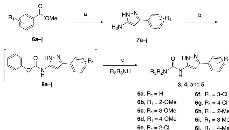
**Scheme 1.** Reagents and conditions: (a) i—LDA, CH<sub>3</sub>CN, THF, −78 °C, 2 h; ii—hydrazine, EtOH, reflux, 5 h; (b) chlorophenylformate, pyridine, rt, 2 h; (c) R<sub>2</sub>R<sub>3</sub>NH, CHCl<sub>3</sub>, reflux, 1 h.
