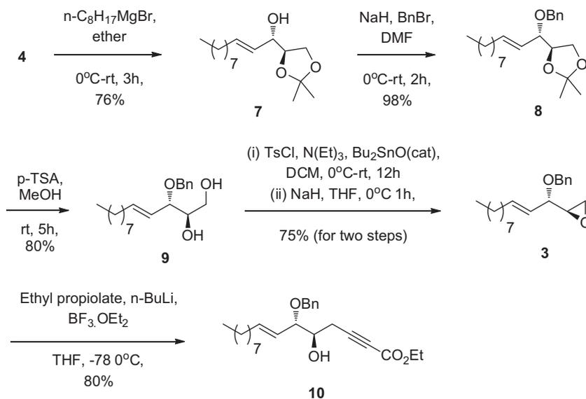
Scheme 3. Synthesis of homo propargylic alcohol intermediate **10**.
