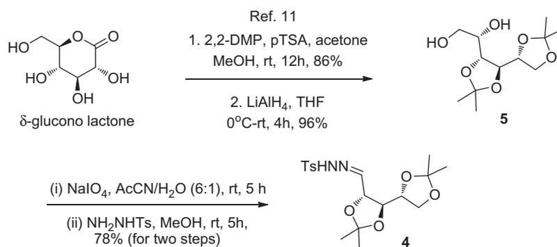
Scheme 2. Synthesis of hydrazone intermediate **4**.
