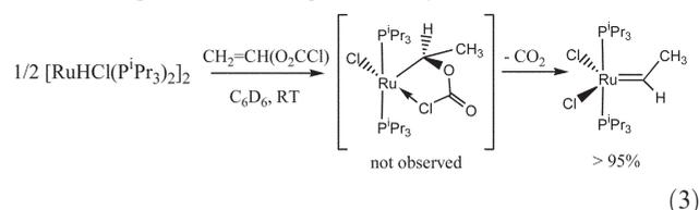
$\text{CH}_2=\text{CH}(\text{O}_2\text{CCl})$ . The combination of these reagents at room temperature (RT) results (eqn. 3) in the immediate, quantitative formation of dichloro carbene,  $\text{RuCl}_2(\text{P}^i\text{Pr}_3)_2(=\text{CHMe})$  and vigorous  $\text{CO}_2$  evolution. We believe this represents a convenient synthesis of this molecule.
