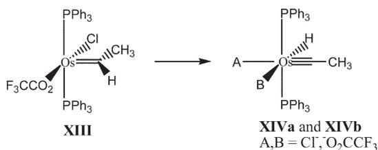
The dichloro-carbene species **XI** spontaneously transforms to its isomeric hydrido-carbyne **XII** analogously to the behavior observed in the reaction between OsHCl(PPh<sub>3</sub>)<sub>3</sub> and vinylchloroformate. The carbyne species **XIVa** then transforms partially to isomeric **XIVb**. The isomer **XIVb** is characterized by a triplet in the hydride region at -7.45 ppm with a  $^2J_{\text{H-P}} = 16$  Hz and a singlet for the carbyne methyl at -0.28 ppm.
