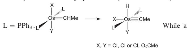
unimolecular 1,2-H migration from C to Os seems an “obvious” mechanism, DFT calculations showed this mechanism to be precluded by a large activation energy (27.2 kcal mol<sup>-1</sup>) in the case where X = Y = Cl.<sup>17</sup>
