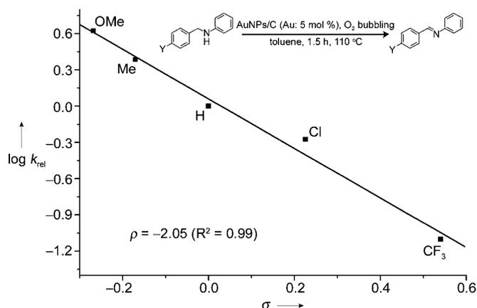
Figure 5. Hammett plot ( $\log k_{rel}$  vs  $\sigma$ ) for the oxidation of *p*-YC<sub>6</sub>H<sub>4</sub>CH<sub>2</sub>NHPH (Y=OMe, Me, H, Cl, and CF<sub>3</sub>) using the “AuNPs/C+O<sub>2</sub>” protocol.
