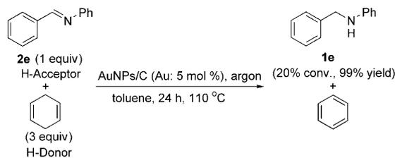
Scheme 8. Hydrogen transfer from donor 1,4-cyclohexadiene to acceptor **2e** catalyzed by AuNPs/C under an argon atmosphere.
