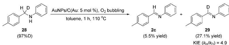
Scheme 4. KIE on the oxidation of **28** by the “AuNPs/C+O<sub>2</sub>” protocol.
