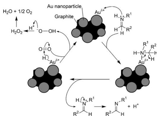
Scheme 5. Proposed mechanism of AuNPs/C-catalyzed aerobic oxidation of amines.
