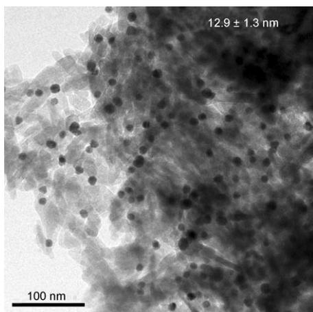
Figure 2. TEM image of the AuNPs/HAP catalyst.
