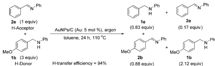
Scheme 7. H-transfer from donor **1b** to acceptor **2e** catalyzed by AuNPs/C under an argon atmosphere.
