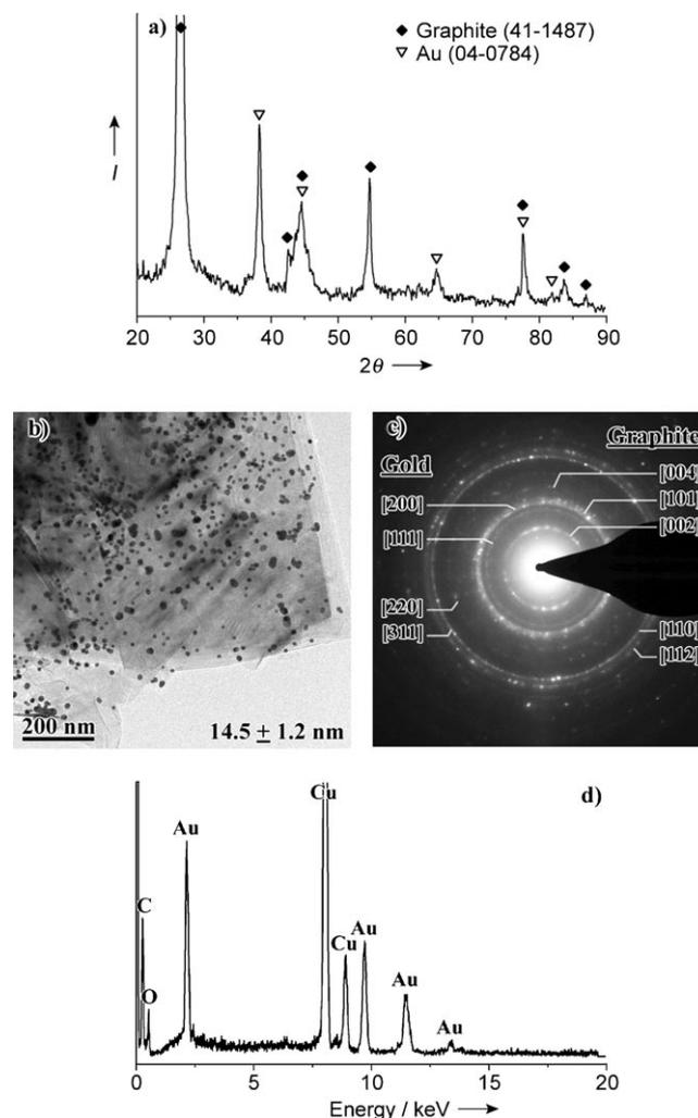
Figure 1. a) Powder XRD pattern, b) TEM image, c) SAED pattern, and d) EDX spectrum of the AuNPs/C catalyst.
