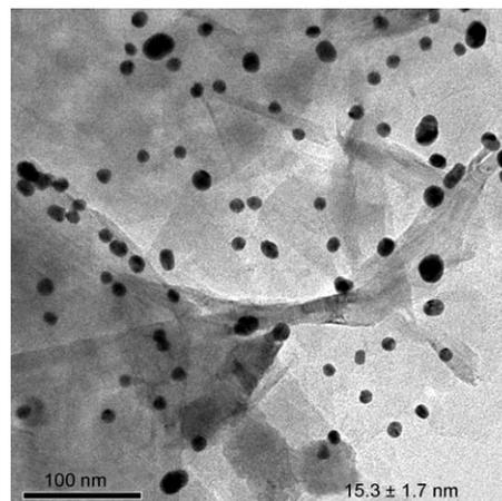
Figure 4. TEM image of the recycled AuNPs/C catalyst.
