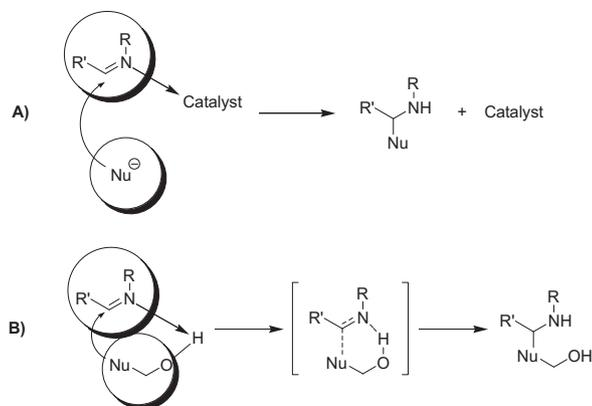
**Scheme 1.** Typical Lewis or Brønsted acid catalyzed system (Path A) versus the proposed self-catalytic system (Path B).
