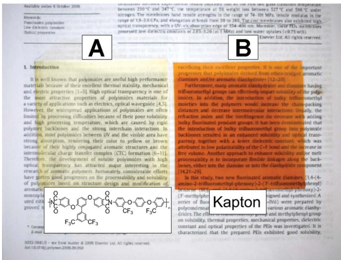
**FIGURE 4** Photographs of a piece of the PEI-4cIII film (89  $\mu\text{m}$  thick) and a piece of the Kapton film (90  $\mu\text{m}$  thick).
