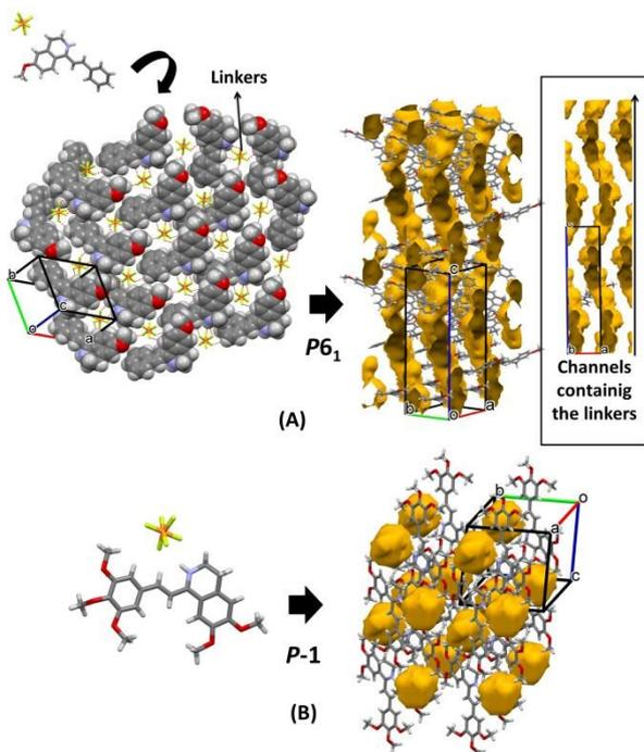
**Fig. 5.** (A) Fluorophosphate ions inside the channels directed along [001] in the enantiomorphic **2a** structure. (B) Fluorophosphate ions inside located voids in 3,4-dihydroisoquinoline-hexafluorophosphate **2b** crystallizing in a centrosymmetric *P*-1 space group.
