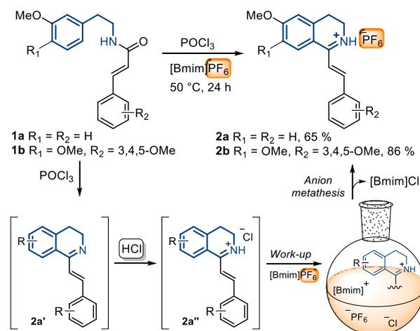
**Scheme 1.** Anion metathesis promoted by the ionic liquid [bmim]PF<sub>6</sub> during the synthesis of dihydroisoquinoline-hexafluorophosphates **2a-b**.
