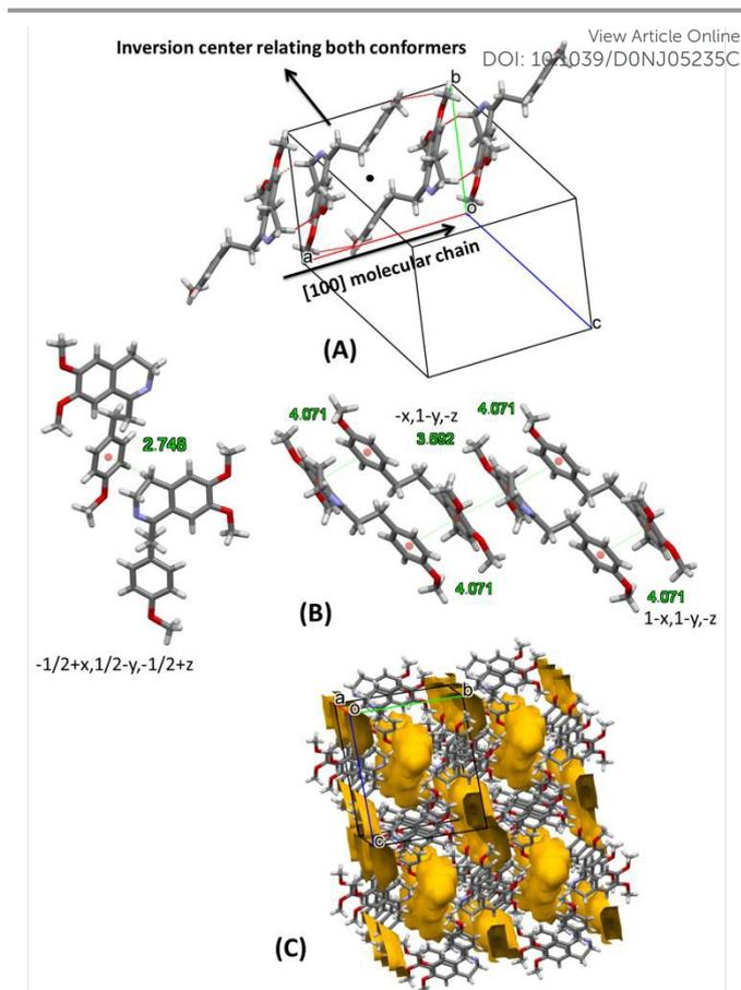
**Fig. 6.** The crystal structure of **2d**, showing (A) the C-H...O (Å), (B) C8-H8A...π and π...π interactions (Å). (C) Voids available for solvent molecules in **2d**.
