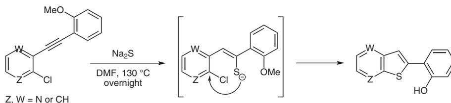
**Scheme 5** Formation of 2-(thieno[2,3-*b*] or [3,2-*b*]pyridin-2-yl)phenols by the reaction of chloro(2-methoxyphenylethynyl)pyridines with Na<sub>2</sub>S<sup>10</sup>
