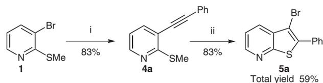
**Scheme 3** Reagents and conditions: (i) PhC≡CH (1.1 equiv), PdCl<sub>2</sub>(PPh<sub>3</sub>)<sub>2</sub> (6 mol%), CuI (3 mol%), Et<sub>3</sub>N (1–2 mL), 100 °C, overnight; (ii) Br<sub>2</sub> (1.5 equiv), anhyd Et<sub>2</sub>O, 0 °C to r.t., 0.5 h, under argon.
