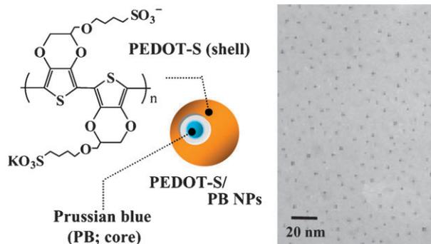
**Fig. 1** (Left) Illustration and (right) TEM image of the prepared Prussian blue nanoparticles protected by the water-soluble  $\pi$ -conjugated polymer PEDOT-S (PEDOT-S/PB NPs).
