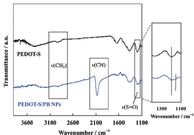
Fig. 2 FT-IR spectra of PEDOT-S and PEDOT-S/PB NPs.
