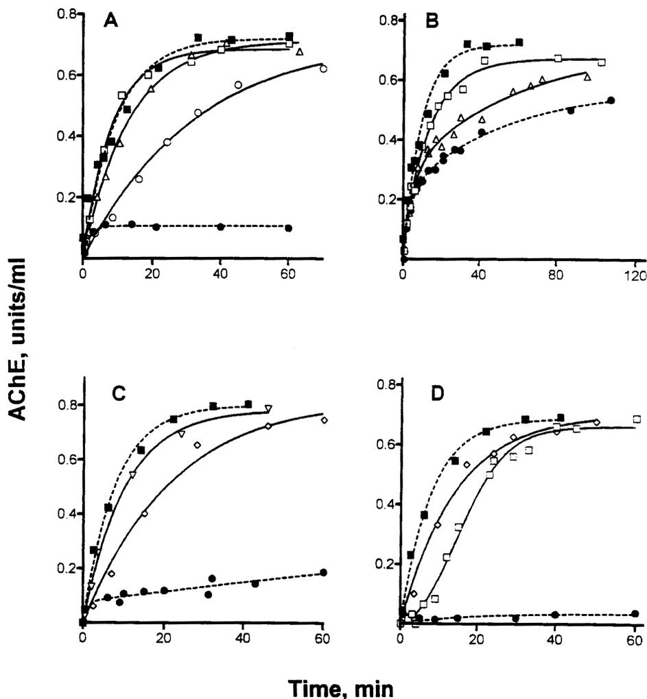
FIG. 3. Time-course of the reactivation of DEP—AChE by 0.2 mM P2S in the presence of 2  $\mu$ M diethylphosphates and various concentrations of OPHps. Dotted lines, controls: (■) no inhibitor, + OPH; and (●) + inhibitor, no OPHs. Solid lines, + inhibitor, + OPHps ( $\mu$ g/mL): (○) 0.01; (△) 0.025; (□) 0.1; (◇) 0.25; and (▽) 1.0. (A) paraoxon; (B) DEFP; (C) TEPP; and (D) DEPQ.
