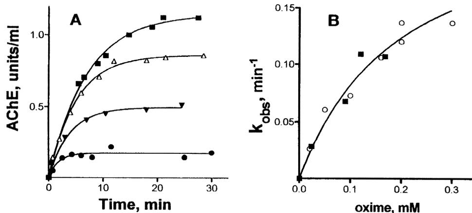
FIG. 2. Reactivation of paraoxon-inhibited AChE. (A) Time—course of reactivation of paraoxon-inhibited AChE by 0.2 mM P2S in the presence of increasing concentrations of paraoxon. Key: (■) no inhibitor; (△) 0.068 μM; (▼) 0.4 μM; and (●) 2.0 μM. (B) Plot of  $k_{obs}$  versus [oxime] for reactivation of paraoxon-inhibited AChE by P2S (○) and its iodide salt, 2-PAM (■).
