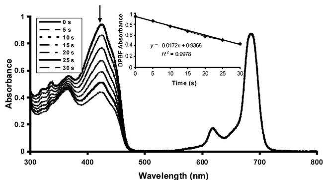
Figure 7. A typical spectrum for the determination of the singlet-oxygen quantum yield. This determination was for compound **3a** in DMSO at a concentration of  $1 \times 10^{-5} \text{ mol dm}^{-3}$ . Inset: plot of DPBF absorbance versus time.
