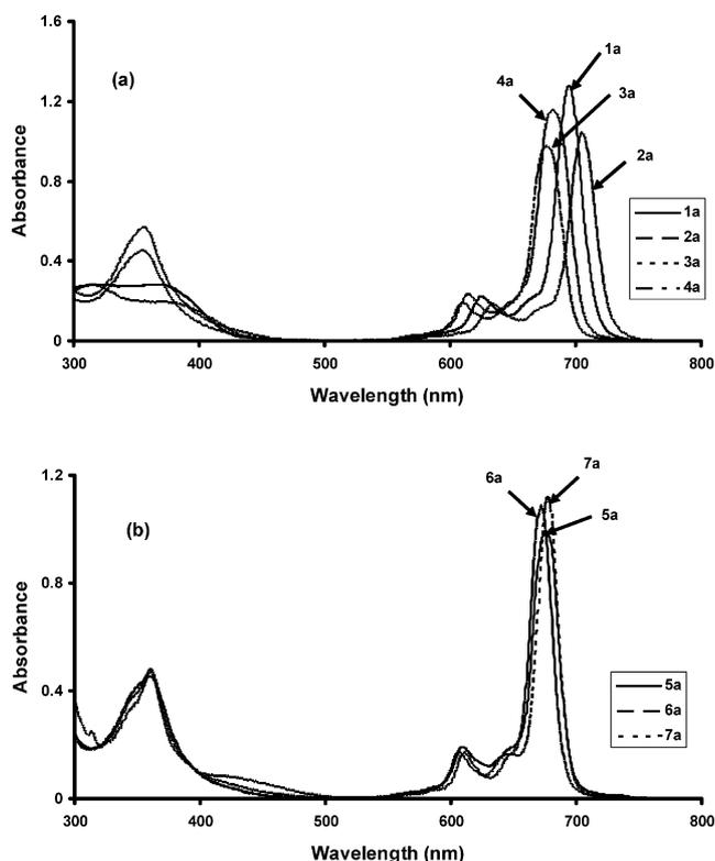
Figure 2. Absorption spectra of (a) tetrasubstituted (**1a**, **2a**, **3a** and **4a**) and (b) octasubstituted (**5a**, **6a** and **7a**) phthalocyanines in DMSO. Concentration: approximately  $4 \times 10^{-6} \text{ mol dm}^{-3}$ .
