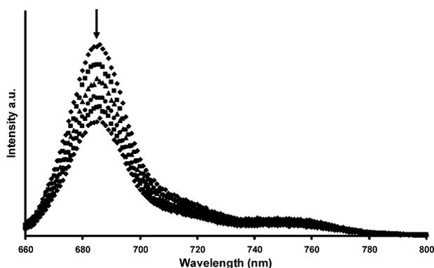
Figure 9. Fluorescence emission spectral changes of **5a** ( $1.00 \times 10^{-5} \text{ mol dm}^{-3}$ ) upon addition of different concentrations of BQ in DMSO. [BQ] = 0, 0.008, 0.016, 0.024, 0.032, 0.040  $\text{mol dm}^{-3}$ .
