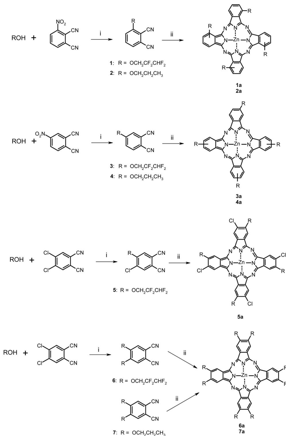
Scheme 1. Chemical pathway used to synthesize the tetra- (**1a**, **2a**, **3a**, **5a**) and octasubstituted (**6a**, **7a**) phthalocyanine derivatives; (i)  $K_2CO_3$ , DMSO, room temperature, 24 h; (ii) *n*-amyl alcohol, DBU, zinc acetate, reflux.
