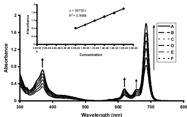
Figure 5. Aggregation behaviour of **7a** in DMSO at different concentrations:  $18 \times 10^{-6}$  (A),  $16 \times 10^{-6}$  (B),  $14 \times 10^{-6}$  (C),  $12 \times 10^{-6}$  (D),  $10 \times 10^{-6}$  (E),  $8 \times 10^{-6}$  (F)  $\text{mol dm}^{-3}$ . Inset: plot of absorbance versus concentration.
