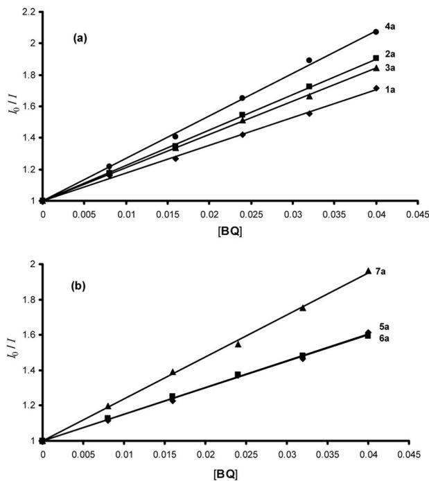
Figure 10. Stern-Volmer plots for benzoquinone (BQ) quenching of (a) **1a**, **2a**, **3a**, **4a** and (b) **5a**, **6a**, **7a**. [MPC] = approximately  $1.00 \times 10^{-5} \text{ mol dm}^{-3}$  in DMSO. [BQ] = 0, 0.008, 0.016, 0.024, 0.032, 0.040  $\text{mol dm}^{-3}$ .
