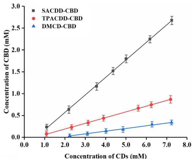
Fig. 2. Phase-solubility diagram of CBD in  $\text{KH}_2\text{PO}_4/\text{K}_2\text{HPO}_4$  buffer solution (pH 7.0, 25 °C) depending on the CDs concentration (SACDD, TPACDD and DMCD).
