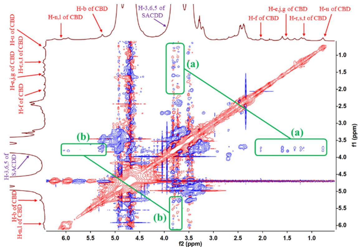
**Fig. 6.** 2D ROESY NMR spectrum for SACDD-CBD inclusion complex in D<sub>2</sub>O: a) cross-peaks between H-f, H-e, H-r, H-s, H-t, H-u protons of CBD and H-3, H-5 protons of SACDD; b) cross-peaks between H-n, H-l, H-b protons of CBD and H-3, H-5 protons of SACDD.
