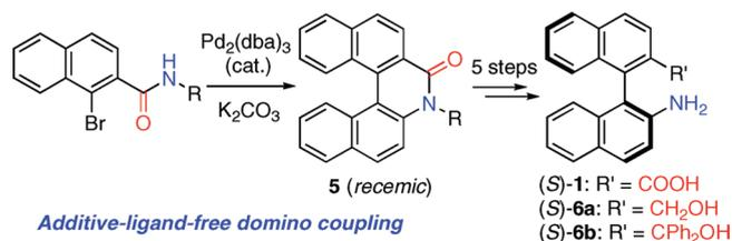
Novel optically active axially chiral amino acid and amino alcohols have been synthesized efficiently via lactam ring-opening, with the aid of an optically active alcohol, amidoaza[5]helicene **5**, which has been readily prepared by an additive-ligand-free Pd catalyzed domino coupling reaction in a single step. The stereostructures of these chiral molecules have also been clarified.
