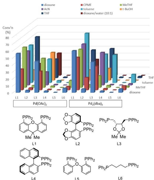
Fig. 3. Subset of HTE results for C–N coupling.
