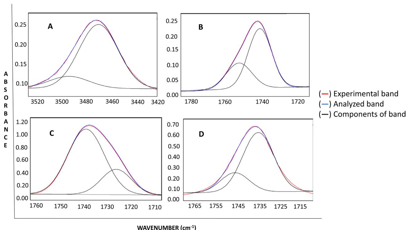
**Fig. 1.** IR analytically resolved carbonyl stretching bands of 2-bromo-2-methylpropyl 2-(4-isobutylphenyl)propanoate **R2**, ibuprofen derivative, in carbon tetrachloride ((A)first overtone and (C)fundamental), chloroform (C) and acetonitrile (D).
