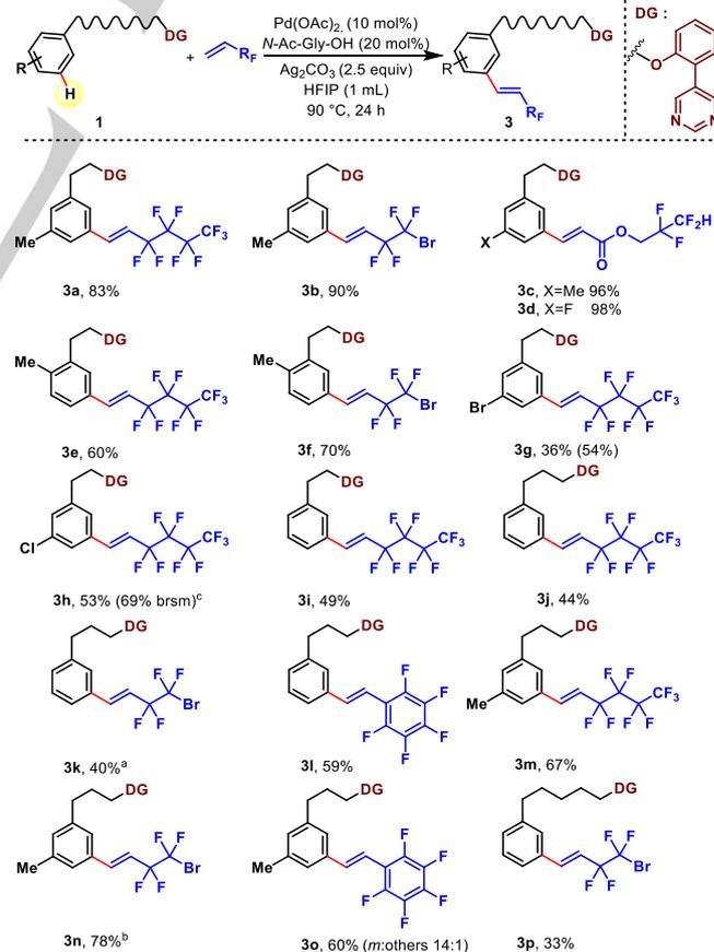
**Scheme 2.** Scope of the *meta*-perfluoroalkenylation with respect to the linker length; <sup>a</sup> reaction was carried out at 70°C; <sup>b</sup> 3 equiv. of olefin were used; <sup>c</sup> brsm
