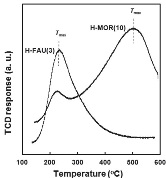
Figure 1. NH<sub>3</sub>-TPD profiles of the zeolite catalysts.
