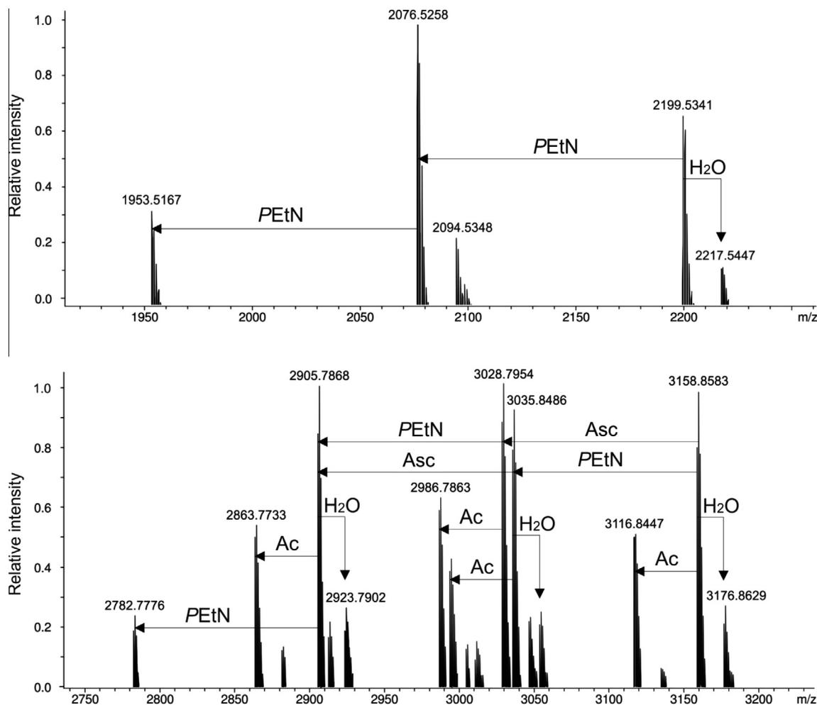
**Figure 2.** Parts of charge-deconvoluted negative ion ESI mass spectra of fractions IIa (bottom) and IIb (top) isolated from the degraded LPS. Shown  $m/z$  values refer to  $[M-H]^-$  ions.
